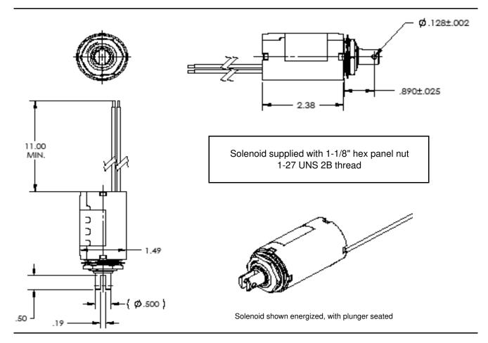
Insulation Materials: UL Construction, Class B 130°C Copper magnet wire insulation rated 155°C (class F)
