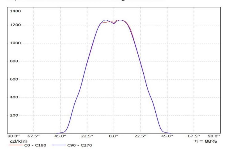
Luminaire: Ledil Oy PRELIMINARY\_F15404\_BARBARA-G2-WW\_+\_F15859\_HEKLA-SOCKET-I\_ (SLE\_G6\_LES15)\_SIMULATED Lamps: 1 x Tridonic SLE G6 LES15 + F15859\_HEKLA-SOCKET-I
