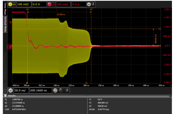
Figure 17. Switching Time Insertion Loss to Isolation
