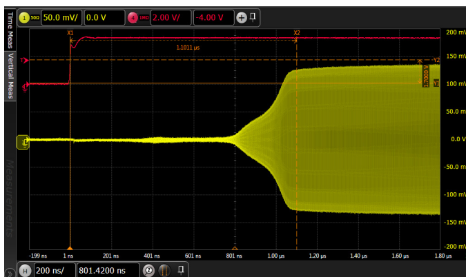
Figure 24. Switching Time [Isolation to Insertion Loss State]
