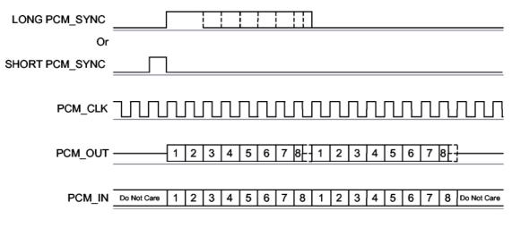
Multi-slot Operation with Two Slots and 8-bit Companded Samples
