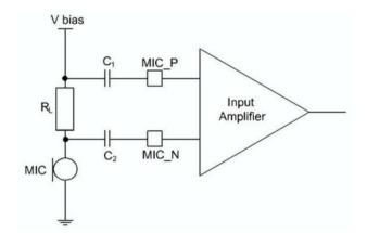
The input impedance at MIC\_N and MIC\_P is typically  $20k\Omega$ . C1 and C2 should be 47nF. R<sub>L</sub> sets the microphone load impedance and is normally between 1 and  $2k\Omega$ . V bias should be chosen to suit the microphone and have sufficient low *noise*. *It may be* obtained by filtering the *output of a PIO* line. (Subject to firmware support, consult available application notes and datasheets or contact free2move)
