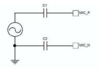
Single-ended Microphone Input (C1 and C2 should be 15nF).
