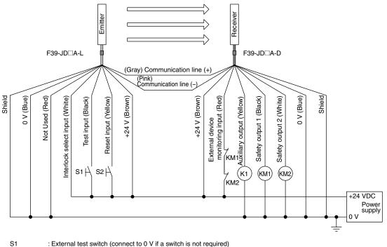
S2 : Interlock/lockout reset switch KM1, KM2 : Safety relay with force-guided contact (G7SA) or magnetic contactor : Load or PLC, etc. (for monitoring) K1
