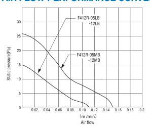
$strule{10}$ The specifications above are typical values measured on the conditions of no-loading running with rated voltage in the circumstances of 25 °C  $\pm$  2 °C, 35~ 85 %RH. Please contact us if you would liketo check the specifications in different circumstances.
