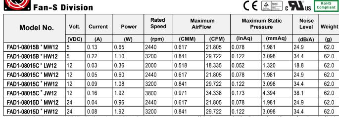
\* Indicates "B" (Ball Bearing), "A" (1B1S), "S" (Sleeve), or "H" (Hydro Dynamic)
