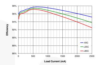
Figure 5. Efficiency vs. Load Current and Input Voltage, V<sub>OUT</sub>=3.15 V
