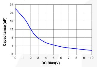
Figure 40. C<sub>EFF</sub> for 22 μF, 0603, X5R, 10 V-Rated Capacitor (TDK C1608X5R1A226M080AC)
