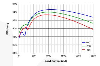
Figure 11. Efficiency vs. Load Current and Input Voltage, V<sub>OUT</sub>=5.0 V
