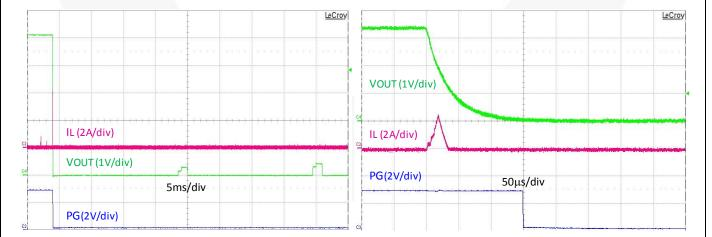
Figure 33. Overload Protection, V<sub>IN</sub>=3.0 V, V<sub>OUT</sub>=5.0 V
