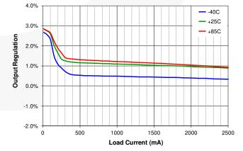
Figure 15. Output Regulation vs. Load Current and Input Voltage, V<sub>OUT</sub>=3.3 V
