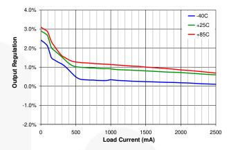
Figure 17. Output Regulation vs. Load Current and Input Voltage, Vout=3.5 V
