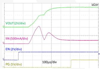
Figure 31. Startup, 50  $\Omega$  Load,  $V_{IN}$ =2.5 V,  $V_{OUT}$ =3.15 V
