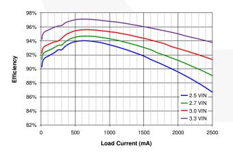
Figure 8. Efficiency vs. Load Current and Temperature, V<sub>IN</sub>=3.0 V, V<sub>OUT</sub>=3.3 V
