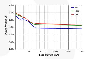
Figure 13. Output Regulation vs. Load Current and Input Voltage, V<sub>OUT</sub>=3.15 V
