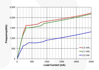
Figure 25. Output Ripple vs. Load Current and Input Voltage, V<sub>OUT</sub>=3.15 V
