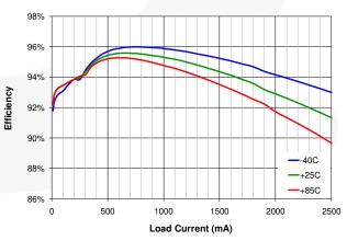
Figure 9. Efficiency vs. Load Current and Input Voltage, V<sub>OUT</sub>=3.5 V
