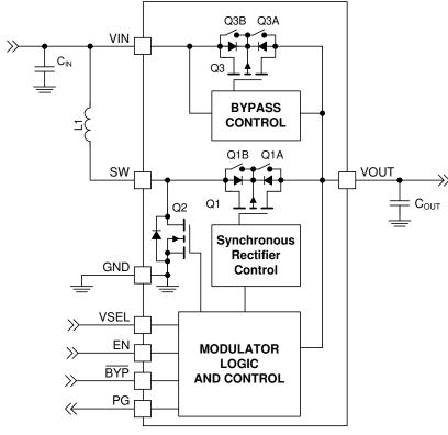
Figure 2. Block Diagram
