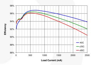
Figure 7. Efficiency vs. Load Current and Input Voltage, Vout=3.3 V
