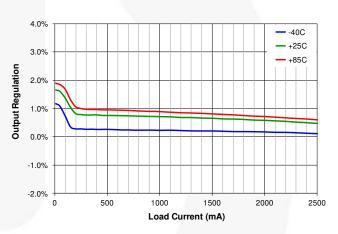
Figure 19. Output Regulation vs. Load Current and Input Voltage, V<sub>OUT</sub>=5.0 V
