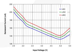
Figure 21. Quiescent Current vs. Input Voltage and Temperature, V<sub>OUT</sub>=3.15 V, Auto Bypass
