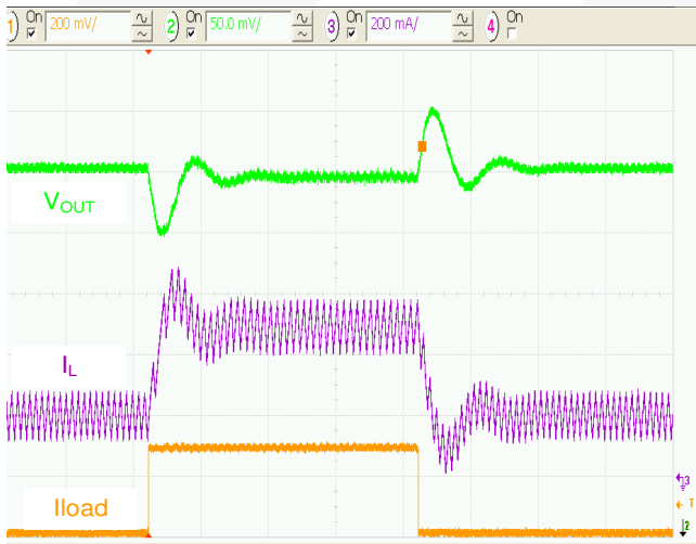
Figure 15. Load Transient 200 to 500mA, 3.6V IN , 5μs/div.
