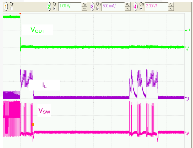
Figure 16. Metallic Short Applied at V OUT , 50μs/div.
