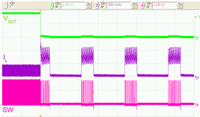
Figure 33. Metallic Short Applied at V_{OUT} , 50\ \mu\text{s}/\text{div.}
