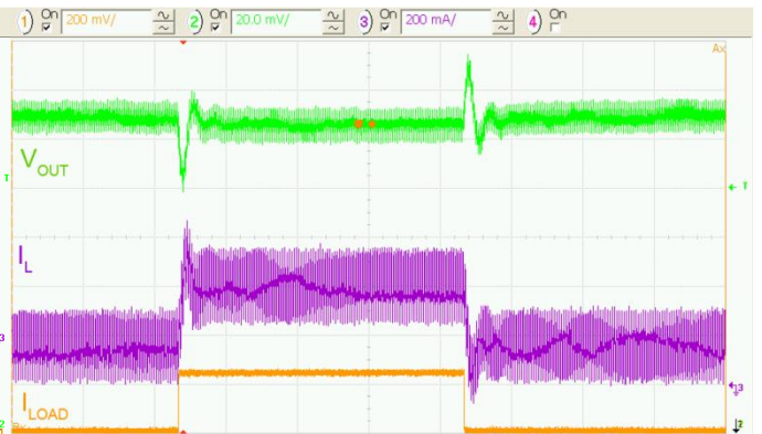
Figure 29. Load Transient 150 to 400 mA, 3.6 V_{IN}
