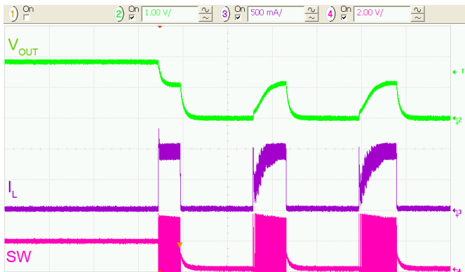
Figure 35. Over-Current Fault Response, R_{LOAD} = 1\ \Omega , 50\ \mu\text{s}/\text{div.}
