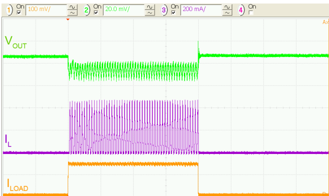
Figure 30. Load Transient 0 to 150 mA, 4.5 V_{IN}
