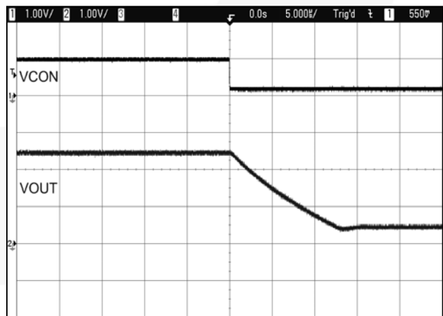
Figure 39. V_{OUT} Falling Transition 3.0 V to 0.5 V, V_{IN} = 3.7\text{ V} in High-Power Mode
