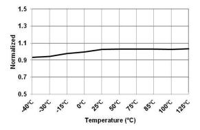
Figure 7. Operating Current Under 5 V ( $I_{\text{IN-OP-LV}}$ ) vs. Temperature
