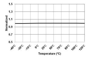
Figure 5.V $_{DD}$  Turn-On Threshold Voltage (V $_{DD-ON}$ ) vs. Temperature
