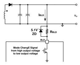
Figure 39. Output Bleeder Function
