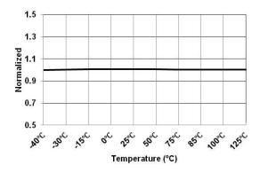
Figure 13. Reference Voltage for CC Regulation at Fixative 1.5 A CC Mode (V<sub>CCR-FIX-1.5A</sub>) vs. Temperature
