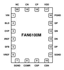
Figure 4. Pin Assignments
