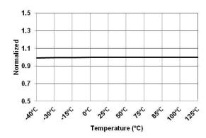
Figure 6.V<sub>DD</sub> Turn-Off Threshold Voltage ( $V_{DD-OFF}$ ) vs. Temperature
