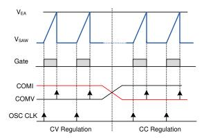
Figure 36. PWM Operation for CV and CC
