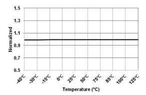
Figure 17. Reference Voltage for CV Regulation at 4 V (V<sub>CVR-4V</sub>) vs. Temperature
