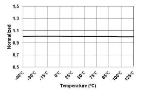
Figure 33. DP Low Level Threshold Voltage (V<sub>DPL</sub>) vs. Temperature
