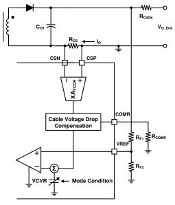
Figure 37. Cable Voltage Drop Compensation Block
