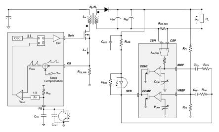
Figure 35. Internal PWM Control Circuit
