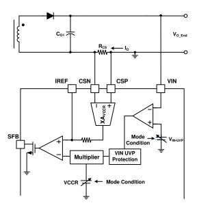
Figure 41. V<sub>IN</sub> Under-Voltage Protection Block
