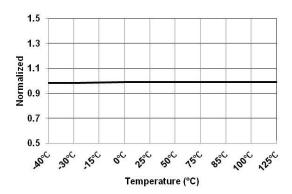
Figure 11. Reference Voltage for CC Regulation at Variable CC 9 V Mode (V<sub>CCR-VR-9V</sub>) vs. Temperature
