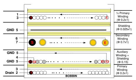
Figure 47. Transformer Diagram
