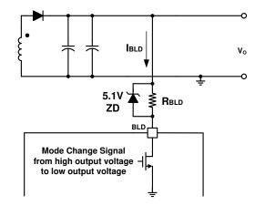
Figure 45. Output Bleeder Function
