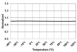
Figure 25.Reference Voltage for CV Regulation at 12 V (V<sub>CVR-12V</sub>) vs. Temperature
