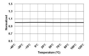
Figure 29. V<sub>IN</sub> UVP Disable Voltage at 9 V (V<sub>IN-UVP-H-9V</sub>) vs. Temperature
