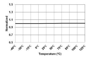
Figure 15. Reference Voltage for CC Regulation at Fixative 2.0 A CC Mode (V<sub>CCR-FIX-2.0A</sub>) vs. Temperature
