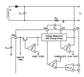
Figure 38. Supply Voltage Block
