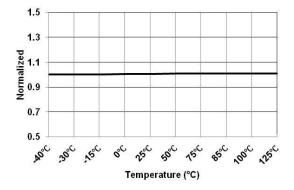
Figure 9. Reference Voltage for CC Regulation at Variable CC 5 V Mode (V<sub>CCR-VR-5V</sub>) vs. Temperature
