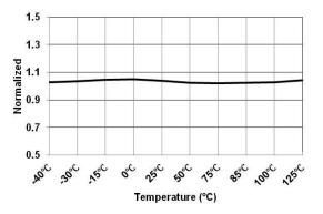
Figure 8. Operating Current Over 5 V (I<sub>IN-OP-HV</sub>) vs. Temperature
