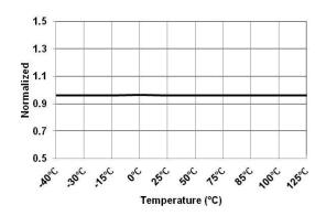
Figure 31.V<sub>IN</sub> UVP Disable Voltage at 12 V (V<sub>IN-UVP-H-12V</sub>) vs. Temperature
