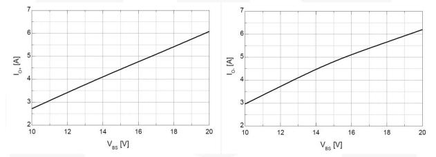
Figure 19. Output High, Short-Circuit Pulsed Current Figure 20. Output Low, Short-Circuit Pulsed Current vs. Supply Voltage vs. Supply Voltage
