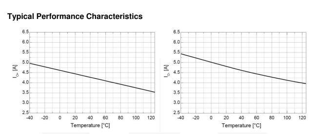
Figure 17. Output High, Short-Circuit Pulsed Current Figure 18. Output Low, Short-Circuit Pulsed Current vs. Temperature vs. Temperature
