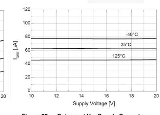
$\label{eq:stable} \begin{array}{lll} \mbox{Figure 22.} & \mbox{Quiescent V}_{BS} \mbox{ Supply Current vs.} \\ & \mbox{Supply Voltage} \end{array}$
