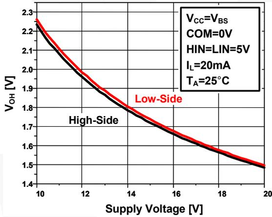
Figure 24. High-Level Output Voltage vs. Supply Voltage
