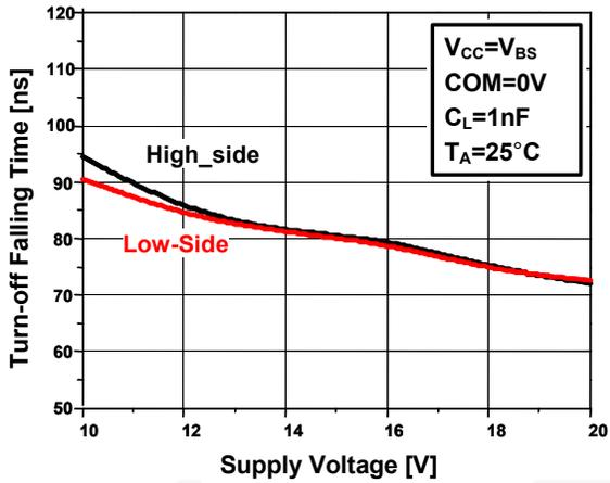
Figure 10. Turn-Off Falling Time vs. Supply Voltage
