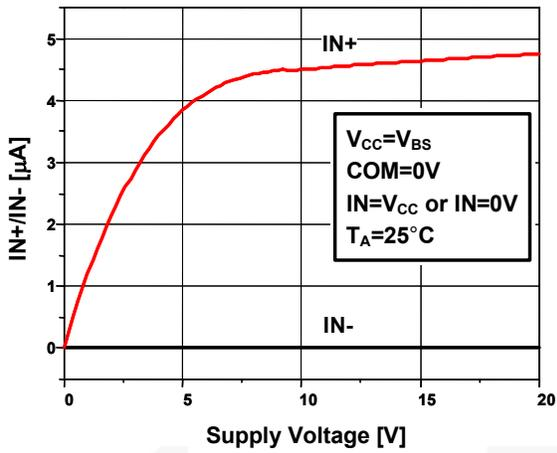
Figure 28. Input Bias Current vs. Supply Voltage
