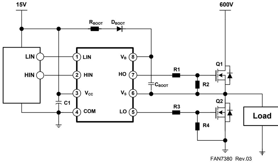
Figure 1. Application Circuit for Fluorescent Lamp Ballast
