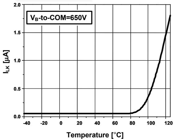
Figure 32.  $V_B$  to  $COM$  Leakage Current vs. Temp.
