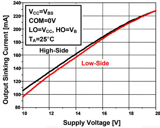
Figure 16. Output Sinking Current vs. Supply Voltage
