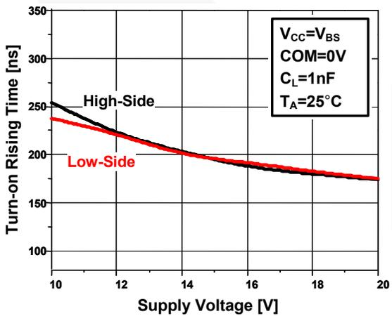
Figure 8. Turn-On Rising Time vs. Supply Voltage
