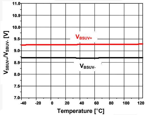
Figure 31.  $V_{BS}$  UVLO Threshold Voltage vs. Temp.
