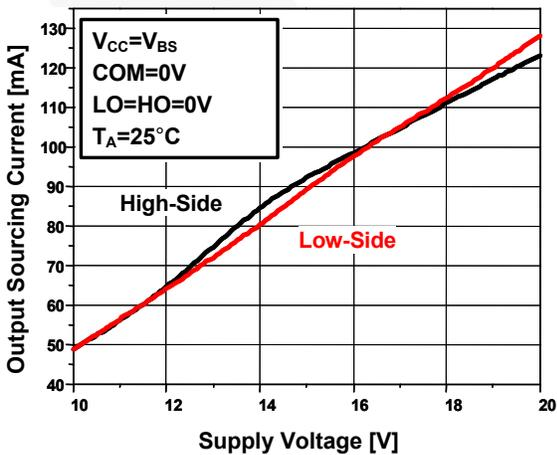
Figure 14. Output Sourcing Current vs. Supply Voltage
