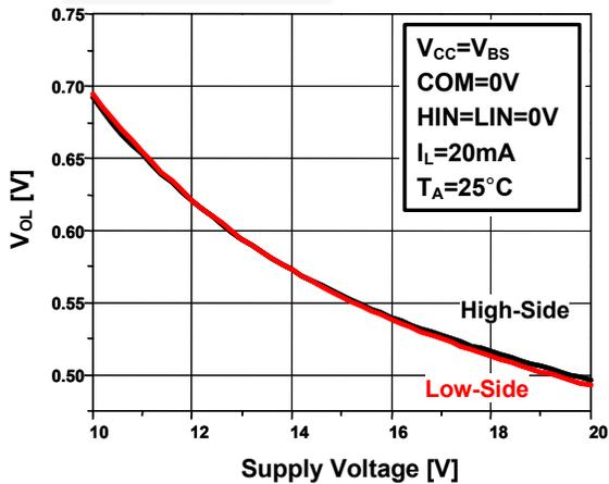
Figure 26. Low-Level Output Voltage vs. Supply Voltage
