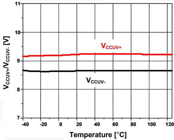
Figure 30.  $V_{CC}$  UVLO Threshold Voltage vs. Temp.
