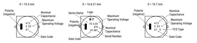
Displays nominal capacitance, maximum operating voltage serial number, polarity, etc.
