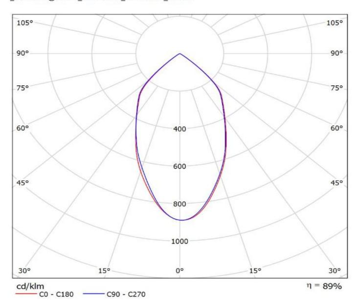
NOTE: The typical divergence will be changed by different color, chip size and chip position tolerance. The typical total divergence is the full angle measured where the luminous intensity is half of the peak value.
