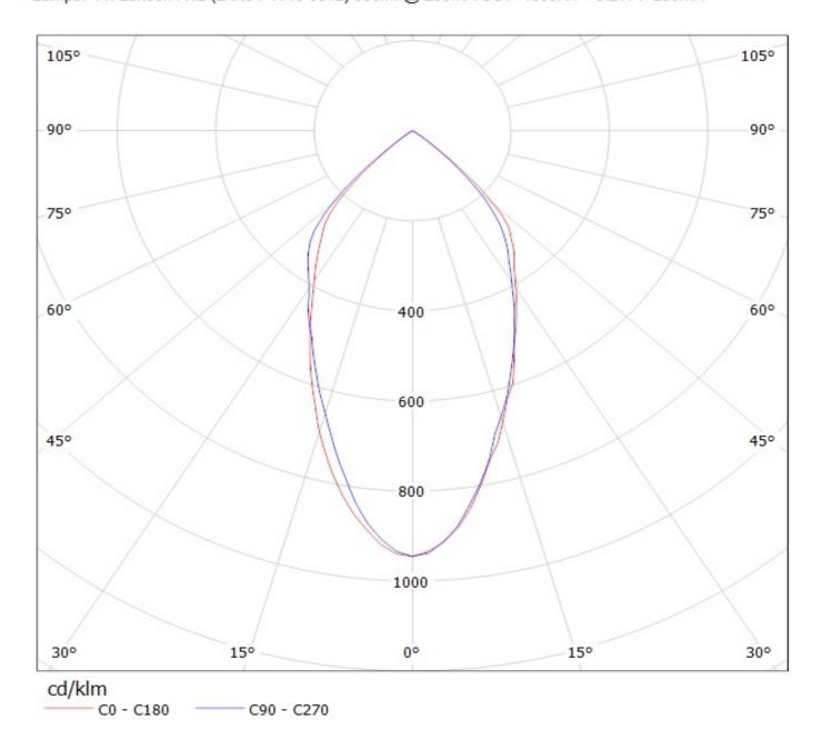
Luminaire: LEDil Oy FC13976\_ANGELINA-RZ-W\_(Luxeon\_K16) Efficiency=89% Lamps: 1 x Luxeon K16 (LXK8-PW40-0016) 1200lm @ 250mA CCT=4000K P=10.9W I=250mA
