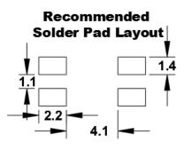
Note: Dimensional drawing is for reference to critical specifications defined by size measurements.
