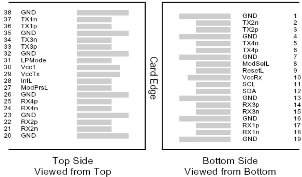
**Figure 1 – QSFP28-compliant 38-pin connector (per SFF-8679)**
