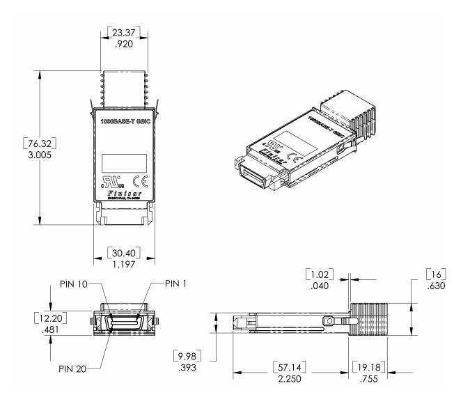
Figure 1. FCL-8520/8521-3 mechanical dimensions
