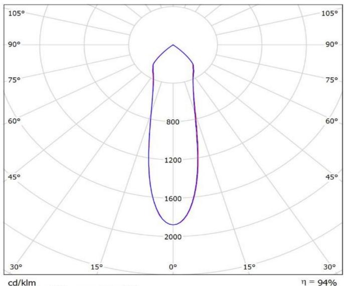
cd/klm - C0 - C180 - C90 - C270 Luminaire: LEDiL Oy FCN13691\_ANGELINA-S\_(Soleriq\_S19)\_462\_Typ\_L3 Lamps: 1 x Osram\_Soleriq\_S19\_(GW\_KAHJB1.EM)\_1497.37lm@250mA\_P=11.1223W\_l=0.2532A
