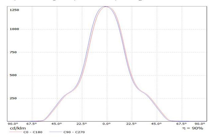
Luminaire: Ledil Oy FCN13691\_ANGELINA-S\_+\_B+W\_434\_TypL1\_BRIDGELUX\_V10\_Gen7\_SIMULATED Lamps: 1 x BRIDGELUX V10 Gen7
