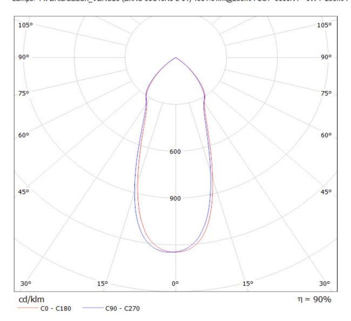
Luminaire: Ledil Oy FCN13691\_ANGELINA-S\_+\_B+W\_434\_TypL1\_BRIDGELUX\_V10\_Gen7\_SIMULATED Lamps: 1 x BRIDGELUX V10 Gen7
