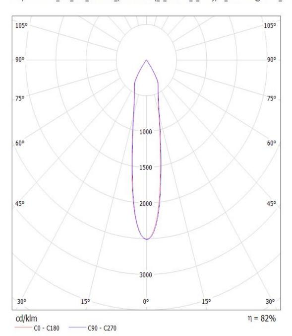
NOTE: The typical divergence will be changed by different color, chip size and chip position tolerance. The typical total divergence is the full angle measured where the luminous intensity is half of the peak value.
