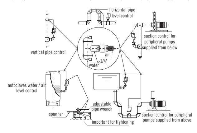
FCNMAS type applications - solution suitable only for pressurised tubing
