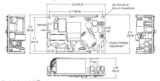
Mounting hole marked with  $\bigoplus$  must be connected to safety earth for class I applications
