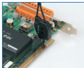
Dully gold-plated surface is detected.
