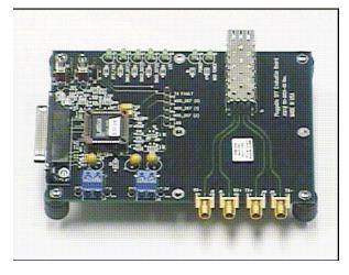
Finisar's FDB-1018 Evaluation Board is the perfect vehicle for testing and evaluating the new Small Form Factor Pluggable (SFP) optical transceivers.
