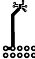
d. 151 °C/W when mounted on a minimum pad of 2 oz copper
