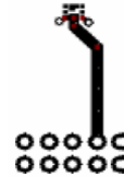
d) 151\text{ }^\circ\text{C/W} when mounted on a minimum pad of 2 oz copper.
