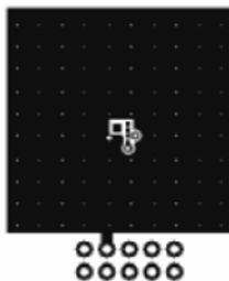
a. 80\text{ }^\circ\text{C/W} when mounted on a 1\text{ in}^2 pad of 2oz copper
