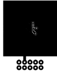
b. 55 °C/W when mounted on a 1 in 2 pad of 2 oz copper
