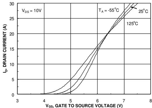
Figure 5. Transfer Characteristics.
