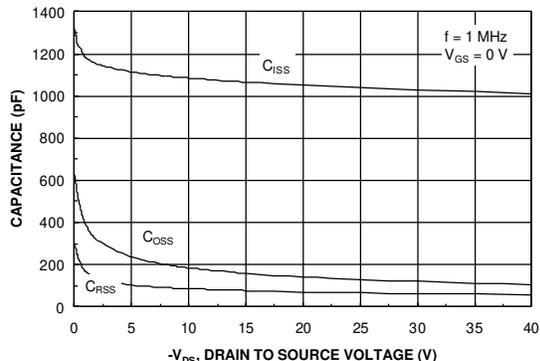
Figure 18. Capacitance Characteristics.
