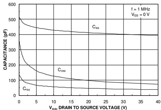
Figure 8. Capacitance Characteristics.
