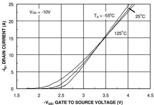
Figure 15. Transfer Characteristics.
