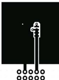
a) 50\text{ }^\circ\text{C}/\text{W} when mounted on a 1\text{ in}^2 pad of 2 oz copper.
