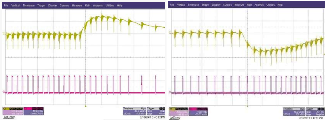
Figure 10. FAN6754AMR+FAN6204MY 230V/50Hz, Overshoot (Ch1: V OUT , Ch2: Gate)
