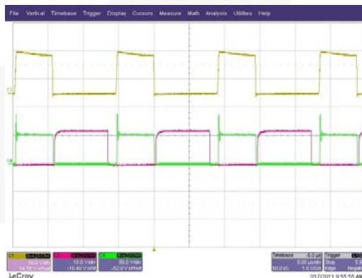
Figure 7. FAN6754WAMR+FAN6204MY, 115 V/60 Hz, 80% Load (Ch1: Gate, Ch2: Gate_SR, Ch4: V dS )
