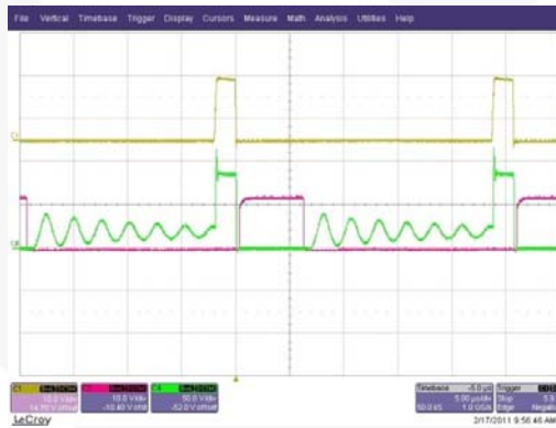
Figure 12. FAN6754WAMR+FAN6204MY 230 V/50 Hz, 20% Load (Ch1: Gate, Ch2: Gate SR , Ch4: V dS )
