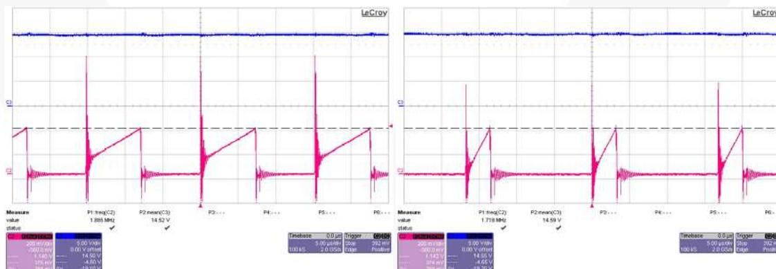
**Figure 22. 90 V / 60 Hz at Maximum Load, Ch1: V<sub>DD</sub>, Ch2: V<sub>CS</sub>**
