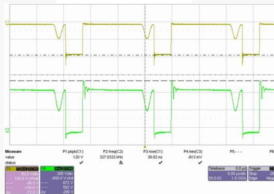
Figure 24. 264 V / 50 Hz at Maximum Load,
