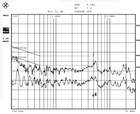
Figure 27. Conduction-Line & Neutral At 115V<sub>AC</sub>
