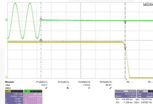
**Figure 10. 264 V / 50 Hz at Maximum Load, Ch1: V<sub>AC</sub>, Ch4: V<sub>O</sub>**
