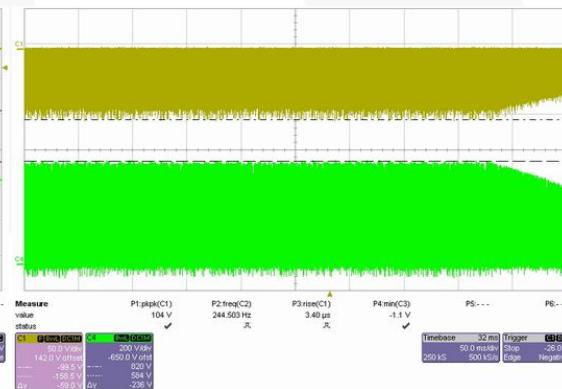
Figure 25. 264 V / 50 Hz at Maximum Load
