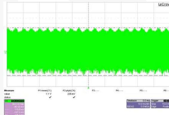
Figure 17. 264 V / 50 Hz at Maximum Load, Ch4:  $V_o$
