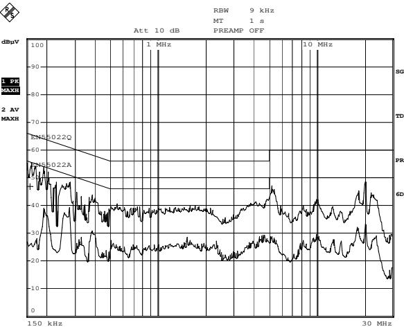
Figure 26. Conduction-Line & Neutral at 115V<sub>AC</sub>
