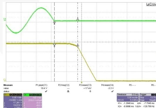
**Figure 9. 90 V / 60 Hz at Maximum Load, Ch1: V<sub>AC</sub>, Ch4: V<sub>O</sub>**
