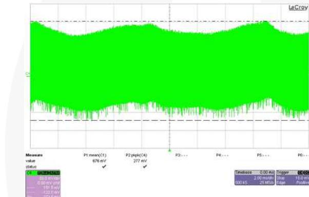
Figure 16. 90 V / 60 Hz at Maximum Load, Ch4:  $V_o$
