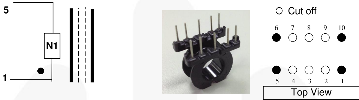
Figure 6. Transformer Specifications of L4
