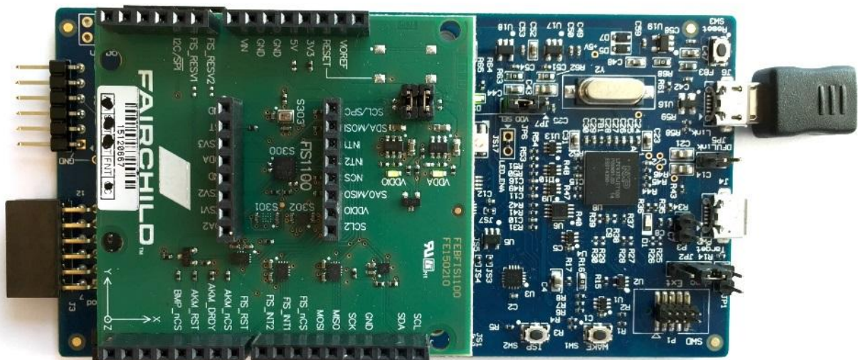
Figure 4. FEBFIS1100MEMS_IMU6D3X Shield Board Mounted on NXP LPCXpresso54102 MCU Evaluation Board
