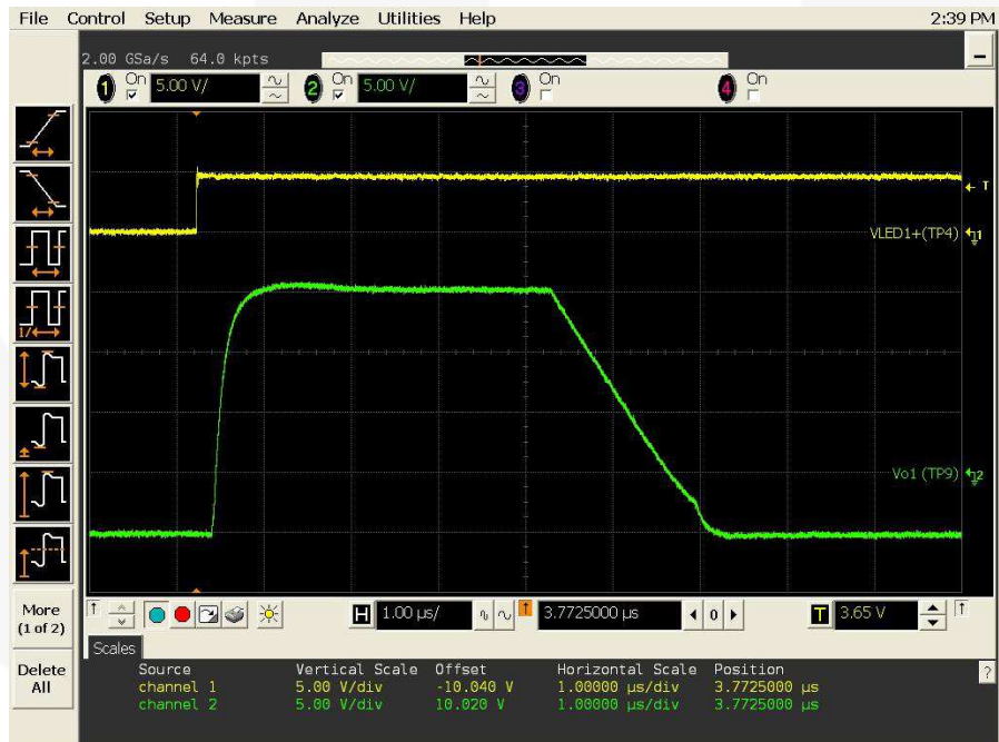
Figure 8. FOD833x without Totem-Pole Current Buffer - V LED1+ and V O1 Waveform During Soft Turn-Off
