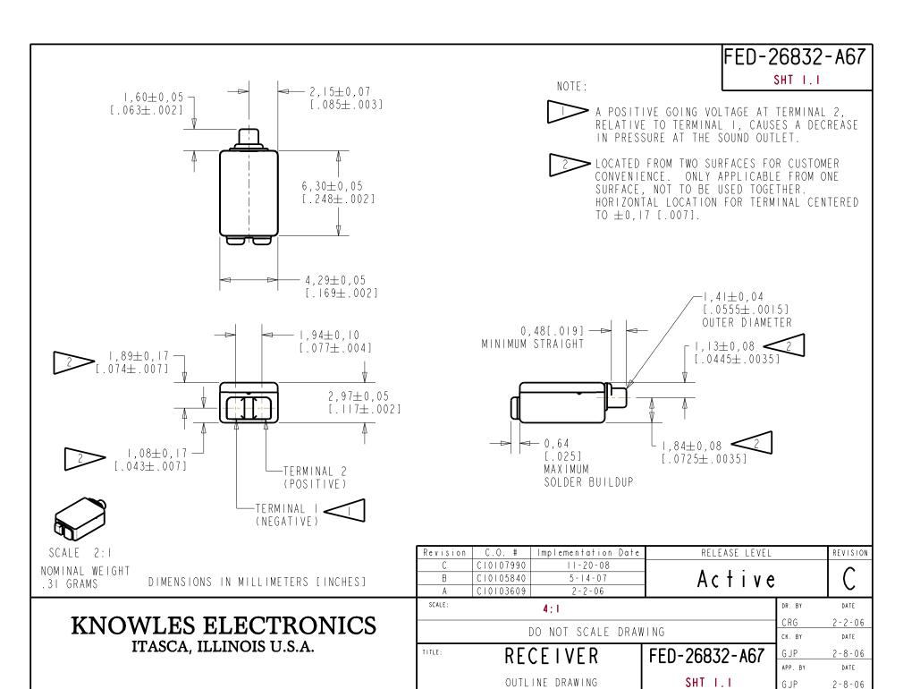
THE FED-26832-A67 IS A FERROFLUID AND TYPE III DAMPED ED
