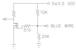
13-1. THE FAN SPEED WILL DEFAULT TO MAXIMUM WHEN THE SPEED CONTROL INPUT IS LEFT UNCONNECTED.
