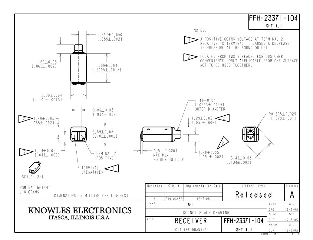
THE FFH-23371-104 IS A FERROFLUID DAMPED FH-23371 RECEIVER WITH A PEAK OF 4dB RELATIVE TO THE SENSITIVITY AT IKHZ UNDER CONSTANT VOLTAGE DRIVE CONDITIONS.
