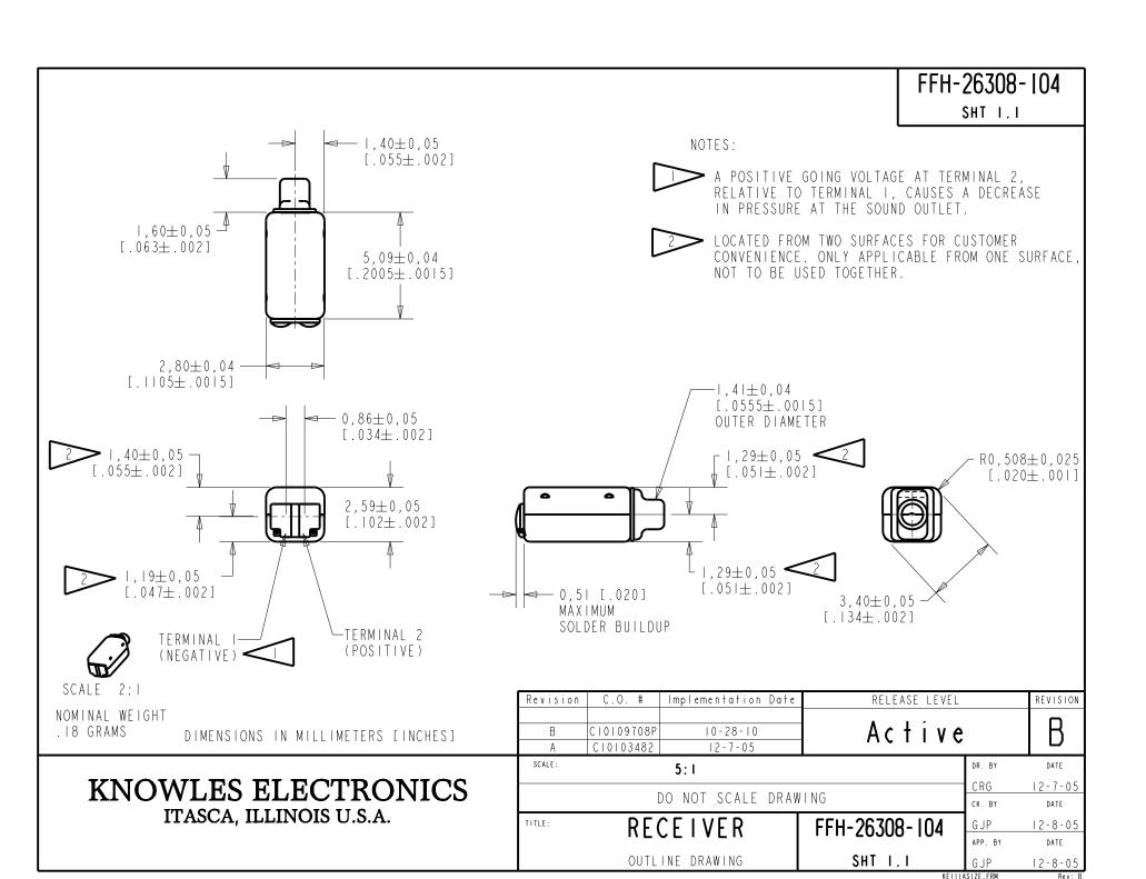
THE FFH-26308-104 IS A FERROFLUID AND TYPE III DAMPED FH-26308 RECEIVER WITH A PEAK OF 4dB RELATIVE TO THE SENSITIVITY AT IKHZ UNDER CONSTANT VOLTAGE DRIVE CONDITIONS.
