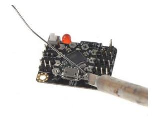
Soldering the Beetle controller on the Beetle shield
