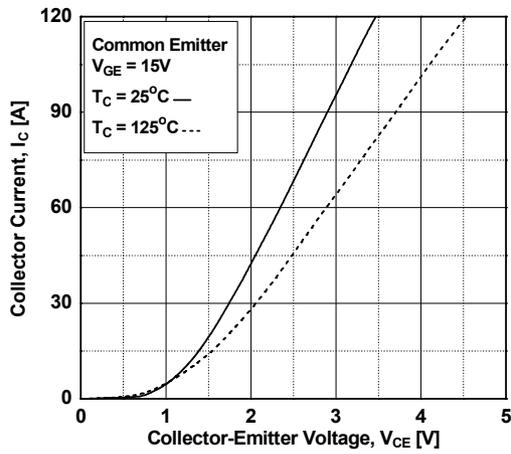
Figure 4. Transfer Characteristics
