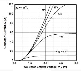
**Figure 4. Transfer Characteristics**
