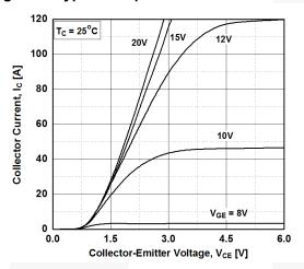
Figure 3. Typical Saturation Voltage Characteristics
