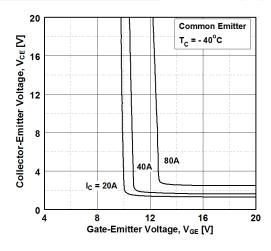
Figure 7. Saturation Voltage vs. V<sub>GE</sub>
