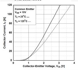
Figure 5. Saturation Voltage vs. Case
