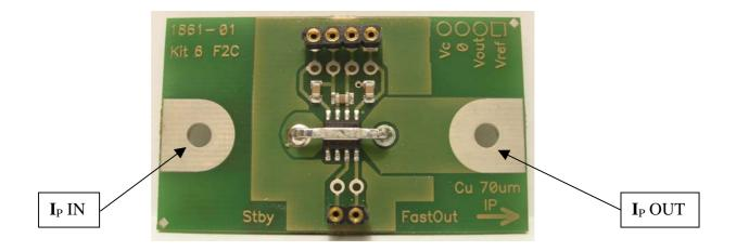
Connect then the primary between pins  $I_P$  IN and  $I_P$  OUT.
