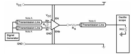
Note A:  $Z_O$  =  $50\Omega$  and  $C_T$  = 15 pF Distributed Note:  $R_L$  =  $100\Omega$  and  $R_S$  =  $950\Omega$
