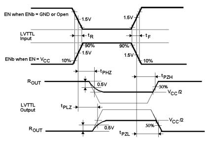
FIGURE 10. LVTTL Output Enable / Disable Timing Waveforms
