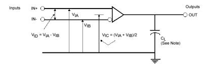
Note:  $C_L = 15 pF$ , includes all probe and jig capacitances
