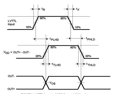
FIGURE 4. LVTTL Input to LVDS Output AC Waveform
