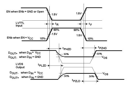
FIGURE 6. LVDS Output Enable / Disable Timing Waveforms
