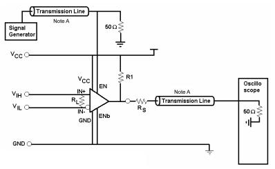
Note A:  $Z_O=50\Omega$  and  $C_T=15$  pF Distributed Note:  $R_L=100\Omega$ ,  $R_S=1000\Omega$ , and  $R_S=950\Omega$
