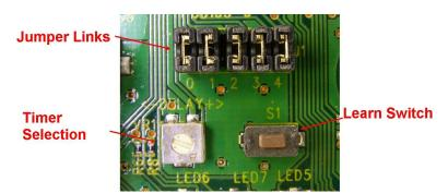
The jumper links configure the outputs to be Momentary, Latching or Timed.
