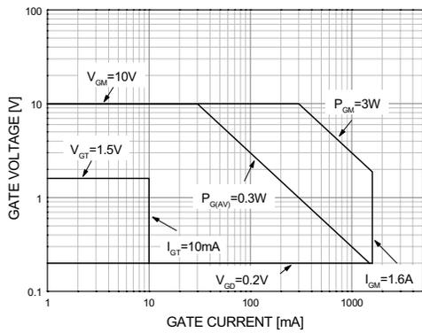
Figure 3. Gate Characteristics
