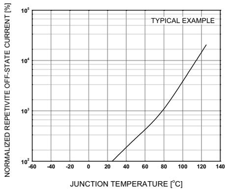
**Figure 9. Repetitive Peak Off-state Current vs Junction Temperature**
