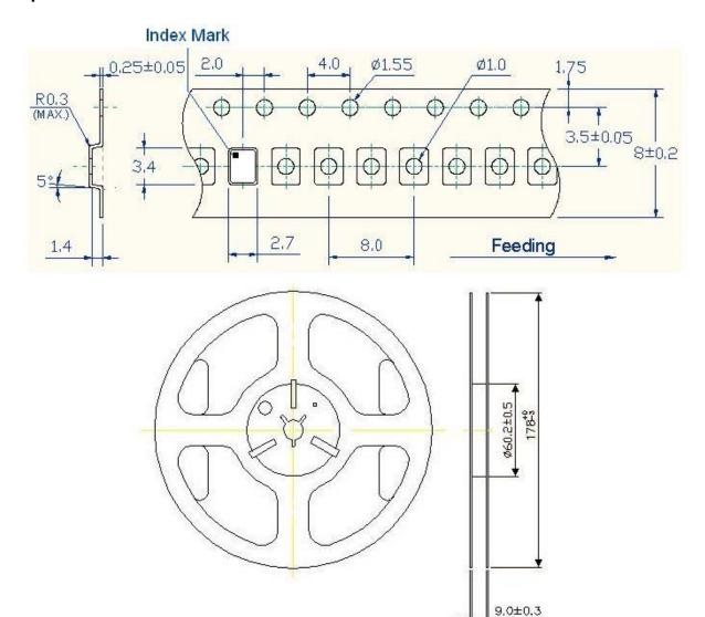
1. 230mm minimum leafer which consist of carrier and/or tape followed by a minimum of 160mm of empty carrier tape sealed with cover tape.
